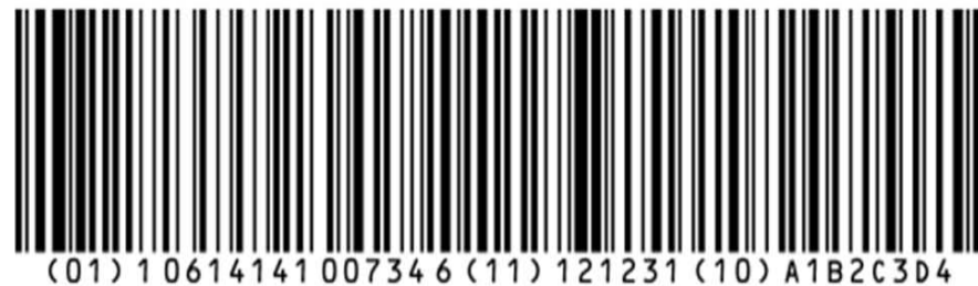
Figure 3. Sample GS1-128 barcode with GTIN (01), Production Date (11), and Batch/Lot Number (10)
